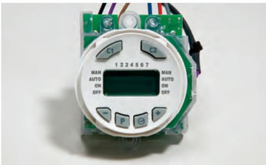
Suits all main heating and hot water needs, when the boiler is connected to a water cylinder. It can be programmed to control the heating and hot water timings at different times each day for a 7 day period.
